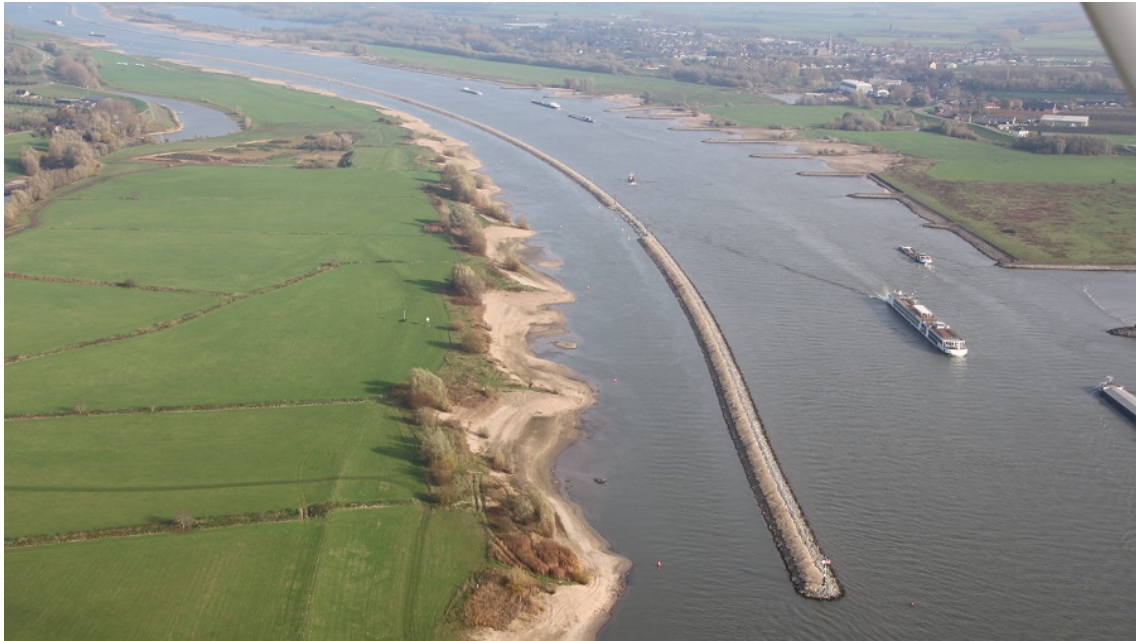
Figure 21 Over a length of 10 km the river Waal is split in two parallel channels, separated by a longitudinal training wall (Photo: Rijkswaterstaat).
